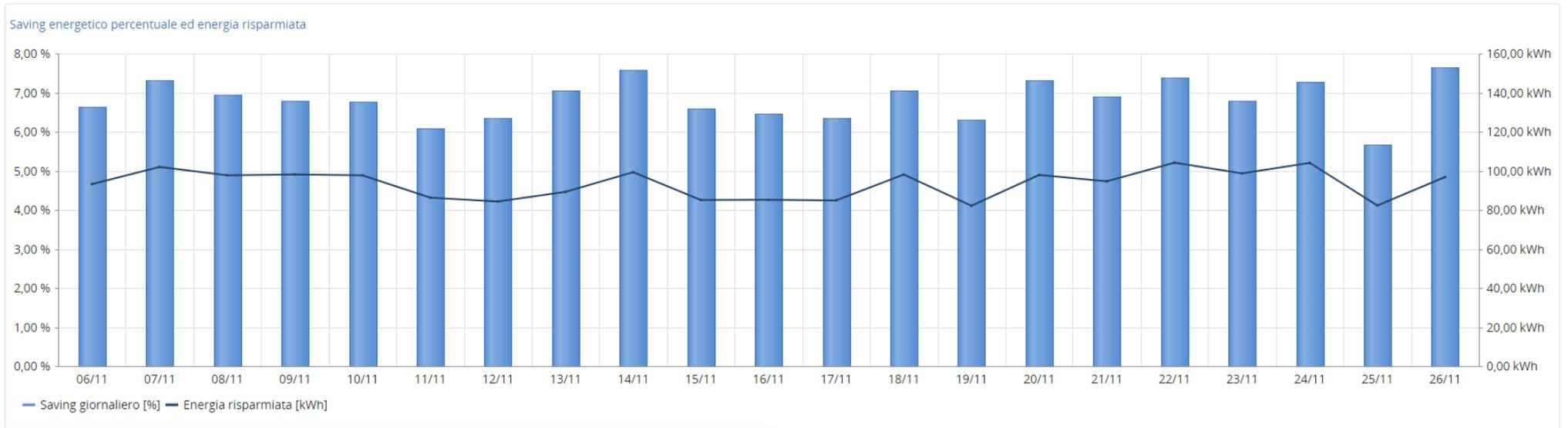
Inside the above graph, we are showing the correlation between the percentages of saved energy over the total absorbed with the actual saved energy.
