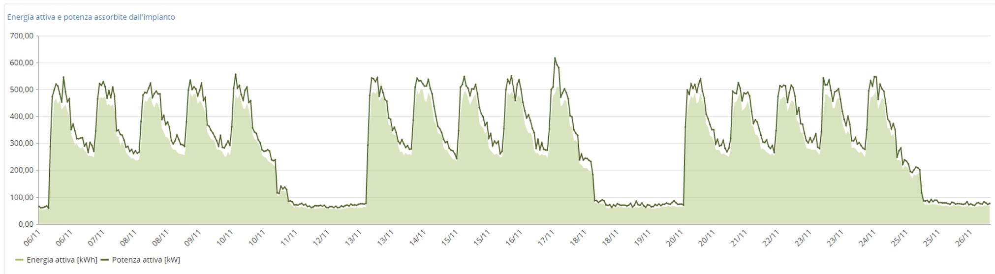
The above graph and curves are showing active energy and power load profiles, absorbed by this plant over a period of 3 weeks.
