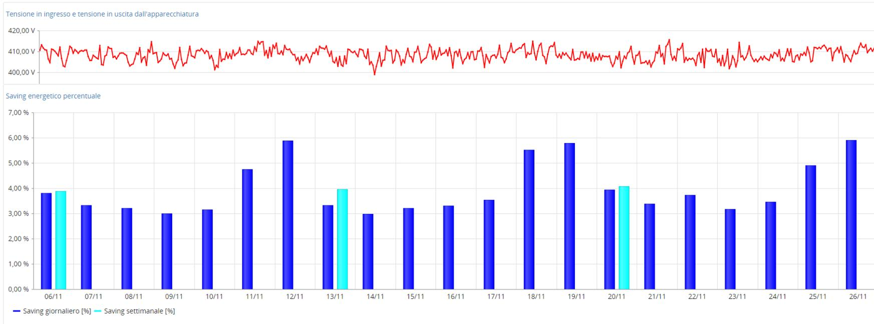
Inside the above graph, that is taken over the same period, it is drawn the incoming voltage profile (mean value is **408,3V**) and the outgoing voltage profile (mean value is **383,9V**). The gap between the voltage profiles allows figuring out the PQL benefits and effects, which are shown in the energy savings. A steady outgoing voltage is also a clear index of a great improvement in a fundamental power quality factor.
