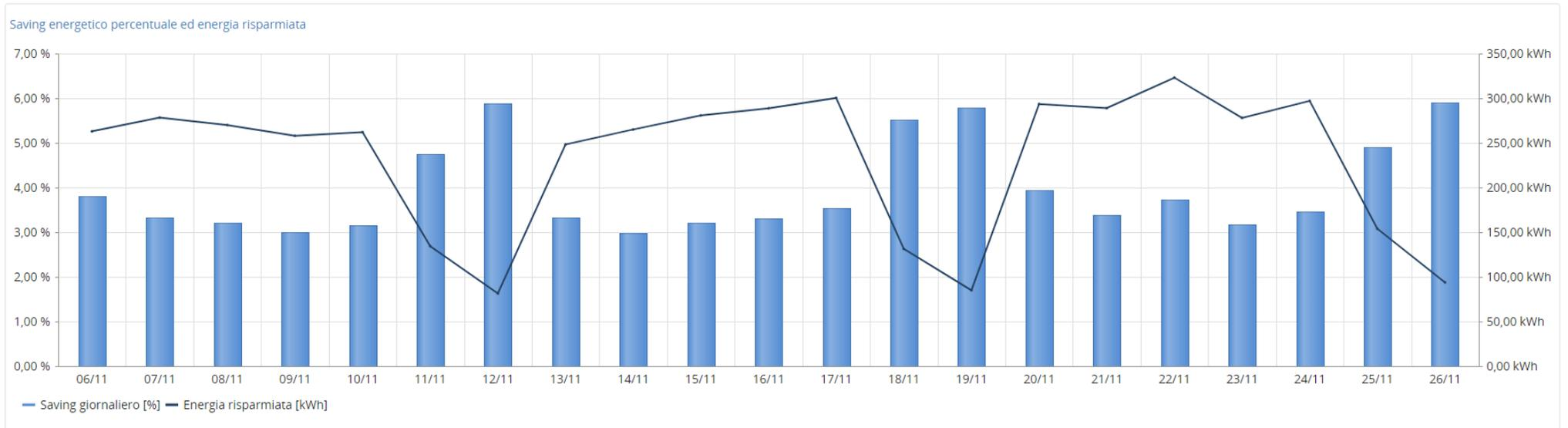
Inside the above graph, we are showing the correlation between the percentages of saved energy over the total absorbed with the actual saved energy. In consideration of what detected over the 3 weeks measuring campaign and what drawn on the graph, it is possible to determine and extrapolate the yearly energy saving, that in this case will be about **80.000kWh**, equivalent to a money saving of **12.000Euro**.
